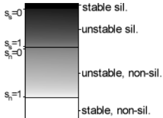
Figure 6: Portrayal of our stability based silhouette coloring scheme. The range of the unstable silhouette and non-silhouette colored areas depend on the thresholds T_s and T_n . Note that s_s = \frac{|N \cdot V|}{T_s} and s_n = \frac{|N \cdot V|}{T_n} .
